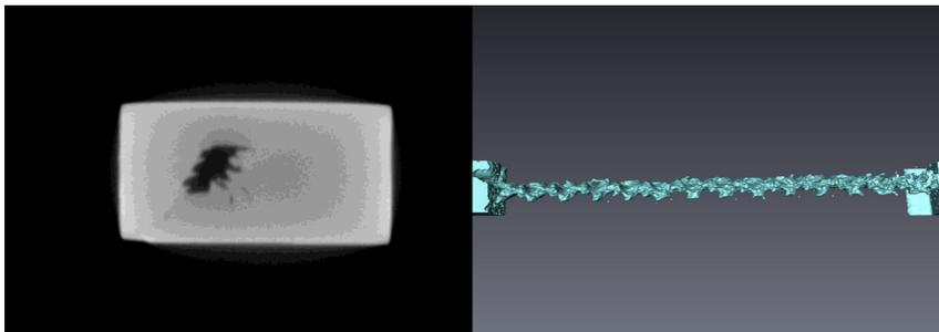
After the a weld is created, X-Ray tomography (left) and computation and computational negation (right) are used to assist with directly interpreting the nature of the weld defect. This gives us the immediate ability to estimate weld integrity.
