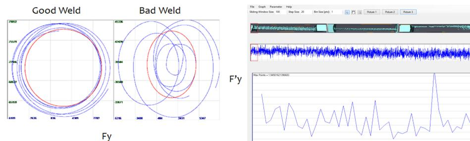
By evaluating phase space analysis of  $F_y$ , and mapping against its own rate of change, a visual representation of a defected weld can be visualized (left). This data supports our hypothesis of material flow being constricted at this particular time stamp – perhaps by temperature of the material.
