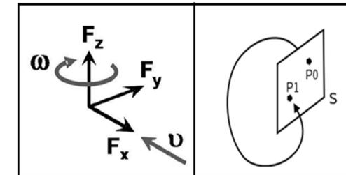
Friction Stir Welding works by traversing a welding tool across butted materials. The direction of the weld,  $F_x$ , Forge pressure,  $F_z$ , and movement into either piece of material,  $F_y$ ,
